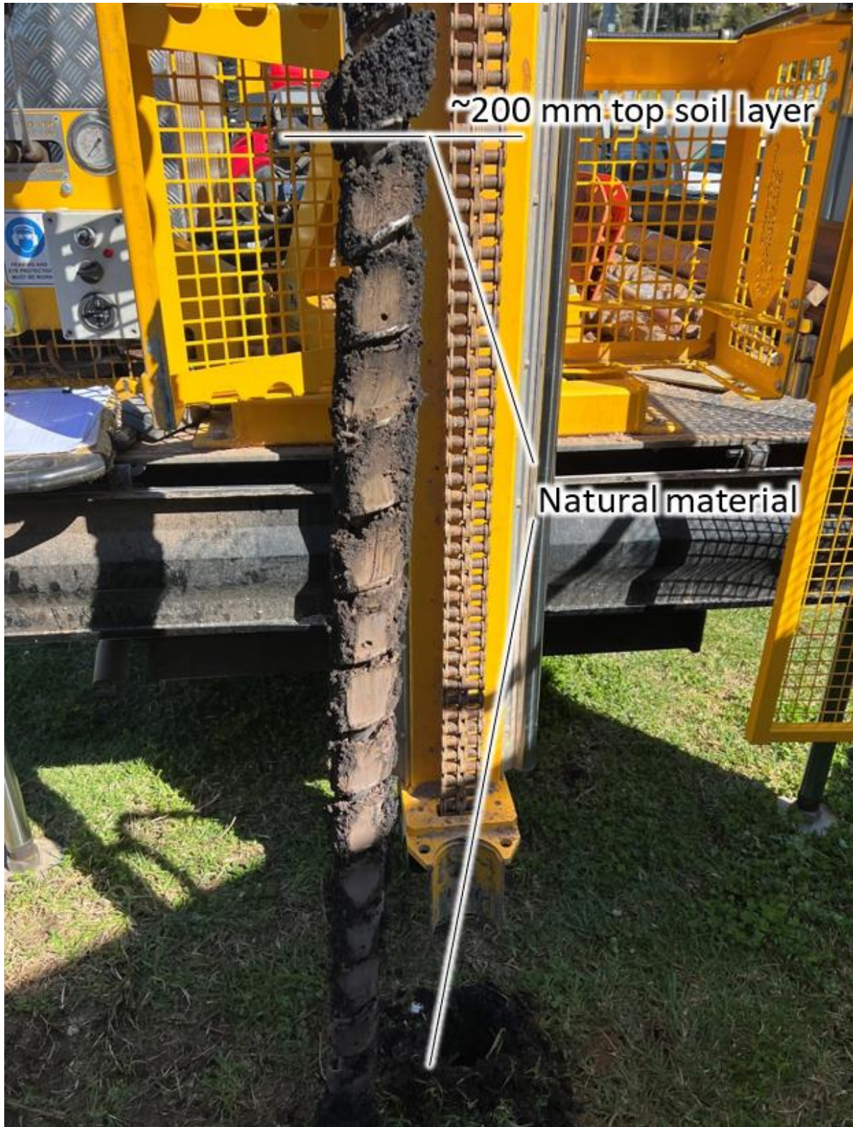
Figure 10c. A ~4 m bore sample, showing ~200 mm of top soil and natural silty clay below that. Sample obtained from the south west corner of the Site. Photo taken 17 Aug 2023.
